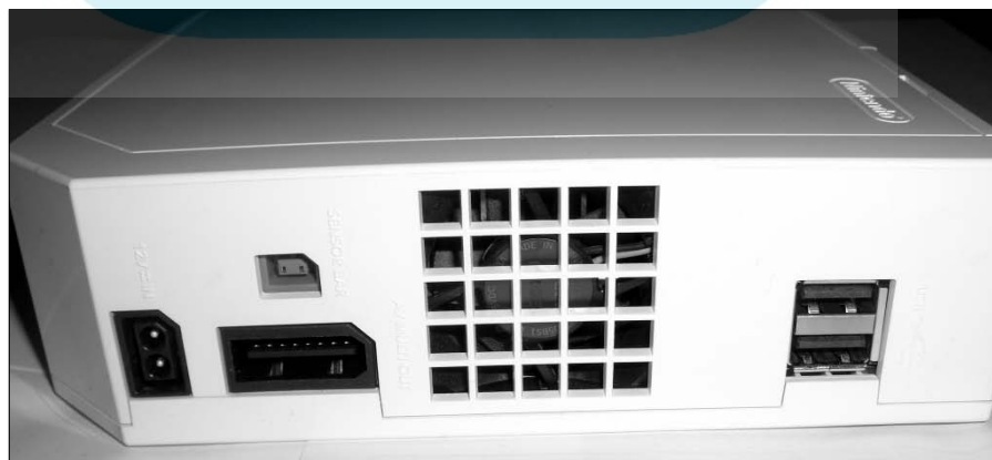
Figure 2-3: The Wii's rear con- nections.
